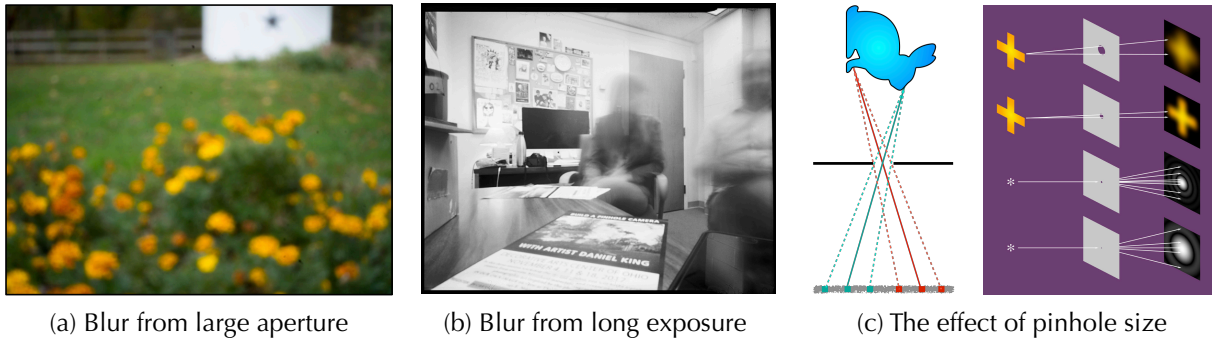
Figure 2: (a): blur from large aperture/pinhole (defocus blur); from Dave Haynie [2019] . (b): blur from long exposure (motion blur); from Daniel King [2017] . (c): defocus blur arises from large pinholes, but when the pinhole becomes very small (on the order of light wavelength) diffraction occurs; adapted from Dominic Alves [2006] .
